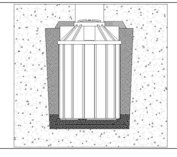
The most suitable PLACE for installation is on a flat surface with compact earth without any recent movements and water sheets and far from foundations or other tanks. **EXCAVATION** creates a hole of approximately 20 cm for the
